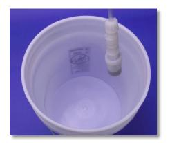
**Step 50:** Place the foot filter into the bucket or stock tank. This ensures the foot filter draws chemistry once you begin operation.
