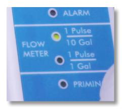
**Step 63:** Press the "**F**" button and select a program to match your water meter. Either 1 Pulse per 1 Gallon (1 GPC), or 1 Pulse per 10 Gallons (10 GPC).
