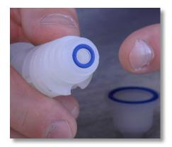
**Step 46:** Grab the filter body and inspect to make sure the small blue o-ring on the top of the filter body is not damaged.
