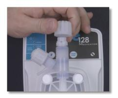
**Step 4:** Locate the discharge valve at the top of the pump head. Remove the discharge valve tube nut, collar, and nozzle. Set all three aside.
