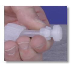
**Step 11:** Push the collar and nozzle together as close as possible.
