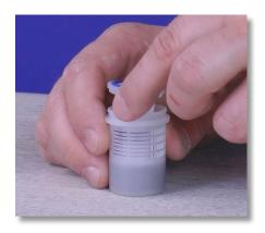
**Step 47:** Set the filter body down, grab the filter basket and put the filter seat back into the filter basket.
