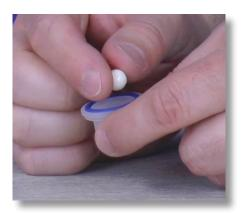
**Step 45:** Put the ceramic ball back into the filter seat and set the filter seat aside.
