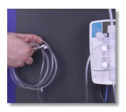
**Step 53:** Using the diagonal pliers, cut the tube so that it is long enough for the chemical bleed off to go into the bucket or stock tank.
