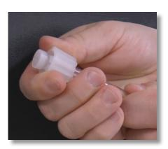
**Step 36:** Slide the tube nut toward the nozzle to compress the collar and nozzle tight together. This should form a ferrule connection.
