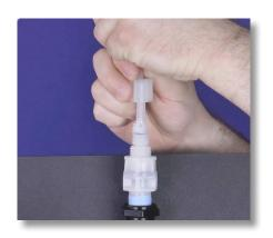
**Step 22:** Attach the tube, and tube connections onto the injection valve by hand tightening the tube nut. Do not cross thread nor overtighten.
