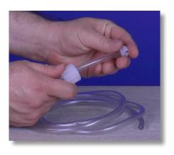
**Step 27:** Slide the collar onto the tube making sure the collar's crown is pointing away from the tube nut.
