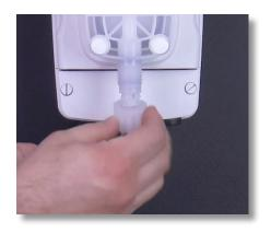
**Step 30:** Attach the tube, and tube connections onto the suction valve by hand tightening the tube nut. Do not cross thread nor overtighten.
