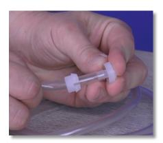
**Step 28:** Take the nozzle and insert the pointed end into the opening of the same tube. Push the collar and nozzle together as close as possible.
