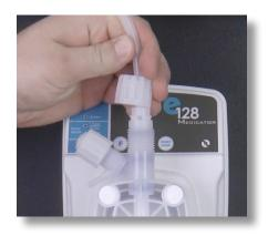
**Step 13:** Attach the tube, and tube connections onto the discharge valve by hand tightening the tube nut. Do not cross thread nor overtighten.
