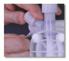
**Step 52:** Locate the manual air bleed barb on the upper left section of the pump's head and slide one end of the PVC tubing over the barb.
