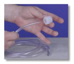
**Step 26:** Slide one end of the PVC tubing through the outside opening of the tube nut.
