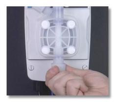
**Step 24:** Locate the suction valve at the bottom of the pump head and remove the suction valve tube nut, collar, and nozzle. Set all three aside.
