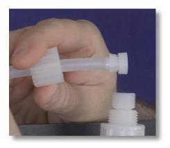
**Step 21:** Slide the tube nut toward the nozzle to compress the collar and nozzle tight together. This should form a ferrule connection.
