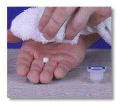
**Step 43:** Set the filter seat down and use the small towel to wipe the ceramic ball clean. Do not misplace it.
