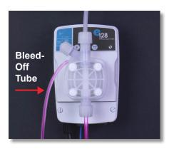
**Step 59:** Once chemical starts going down the bleed-off tube, close the air bleed valve on the pump's head.
