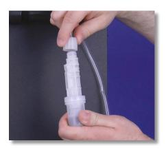
**Step 49:** Grab the PVC suction tubing hanging down from the suction valve; and attach tube, foot filter tube nut, collar, and nozzle onto the foot filter by hand tightening the tube nut. Do not cross thread nor overtighten.
