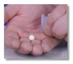
**Step 42:** Pour the ceramic ball out of the filter seat and into your hand.
