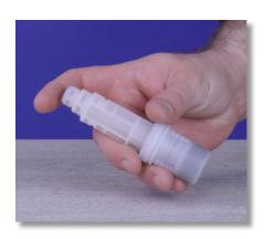
**Step 38:** Grab the foot filter and shake it back and forth. You should hear a ceramic ball moving freely inside.
