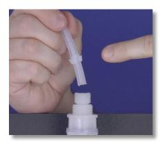
**Step 19:** Slide the collar onto the tube, making sure the collar's crown is pointing toward the injection valve.
