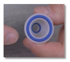
**Step 44:** While holding onto the ceramic ball, inspect the two blue o-rings in the grooves of the filter seat and make sure they are not damaged.
