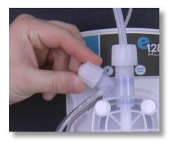
**Step 57:** Open the air bleed valve on the top left of the pump's head and push the **Start/Stop** button.
