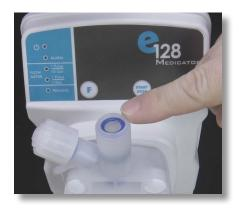
**Step 7:** Make sure not to lose the o-ring directly underneath the transit washer.
