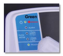
**Step 61:** When the priming process completes, the **e128 Medicator** stops stroking and the power LED lights up green.
