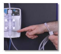
**Step 37:** Let the PVC suction tubing, along with the foot filter tube nut, collar, and nozzle hang from the pump head.
