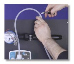
**Step 17:** Grab the rigid polyethylene discharge tube connected to the discharge valve. Using diagonal pliers, cut the tube so that it runs comfortably from the discharge valve to the injection valve.
